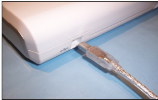
Connect the Type B plug to the rear of the Electronics Module
